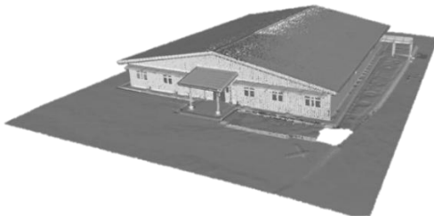
Picture 2 TLS result Point Cloud
