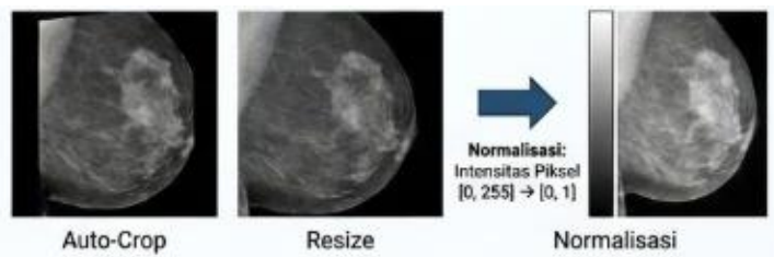
Figure 1. Details of Image Pre-Processing Transformation Stages
